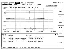
Example of measurement result of gain FN of EDFA
